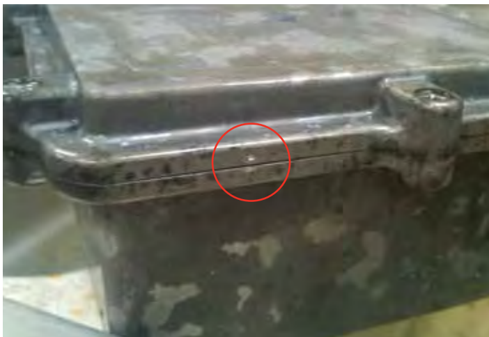
FIGURE 7: ENCLOSURE VISUALLY INSPECTED AFTER THE TESTING
