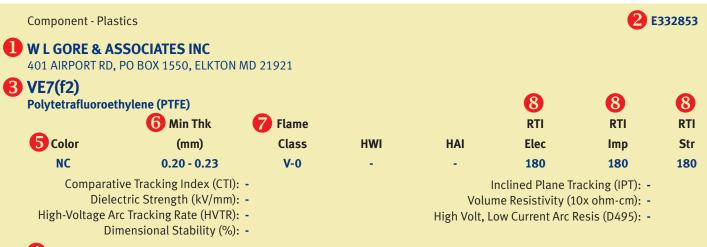
(f2) - Subjected to one or more of the following tests: Ultraviolet Light, Water Exposure or Immersion in accordance with UL 746C, where the acceptability for outdoor use is to be determined by UL.
