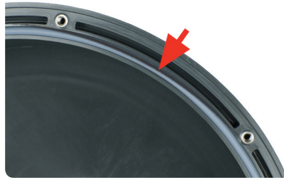
Figure 2. Failed Seal in a GPS System
