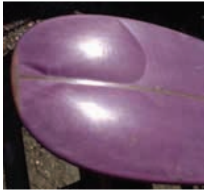
▲ Bubble trouble: Surface layer delamination caused by thermal expansion of EPS. ▼ Pressure relief: A Gore ePTFE vent is open to air; closed to water, salt, and sand.
