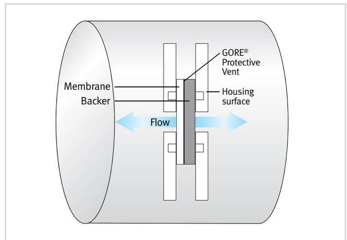
**FIGURE 4: SCREW-IN VENT POSITION DURING AIRFLOW TEST**
