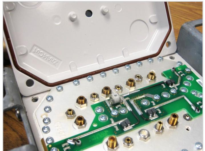
Visual inspection of the vents identified that four were compromised. Because there was no evidence of damage to the electronics or housings in which these vents were installed, the damage most likely occurred during or after the equipment was removed from service.
