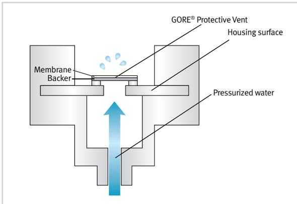
**FIGURE 6: SCREW-IN VENT POSITION IN WATER PRESSURE TESTING EQUIPMENT**
