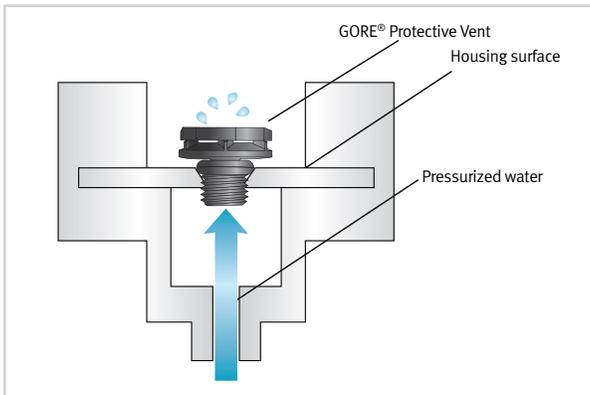
1. Water pressure was maintained at approximately 103 mbar to simulate 1 meter of water submersion, as required by the Ingress Protection level of IPX7.
