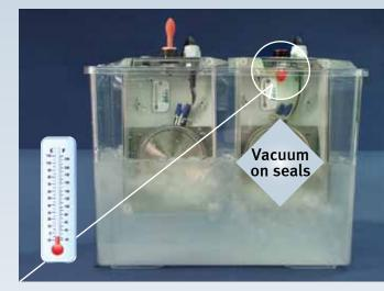
The drastic temperature change causes a vacuum, drawing the balloon into the enclosure. In a real-world situation, contaminants such as liquid, dirt and particles can be drawn into a device, causing failure to internal components.
