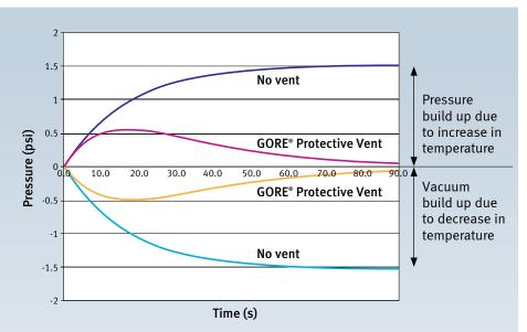
When exposed to rapid heating and cooling cycles, the enclosure without a vent builds up pressure (see positive pressure build on graph) and a vacuum (see negative pressure build on graph). Conversely, an enclosure vented with a GORE<sup>®</sup> Protective Vent maintains equalized pressure with its environment.
