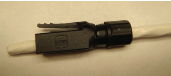
Figure 5: Attaching the labels, sleeving and black housing
